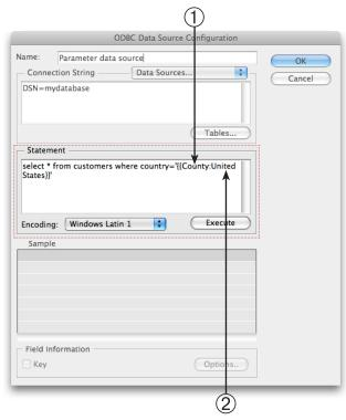
Parameters are included in the SQL statement inside of {{ brackets }}. ① The value inside of the brackets is the name of the parameter presented to the user; ② a default value can also be included.
